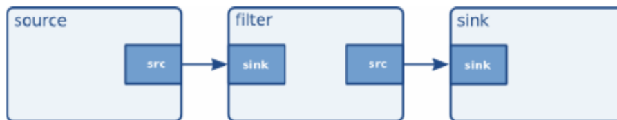
Figure 4.2: A Model GStreamer Pipeline
